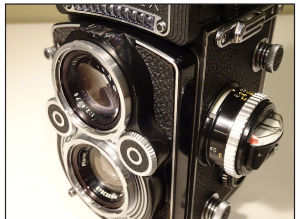
Close-up of a later Rolleiflex 3.5F showing aperture and shutter speed controls (on either side of the lenses) and coupled match needle metering dial inside the focusing ring on the camera body’s side. The exposure system was easy to use and worked well.
