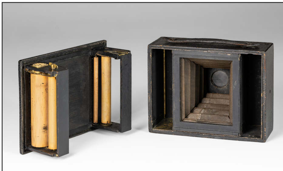
Figure 2: Rear view of camera showing how the integrated roll-film back fits into the body.
