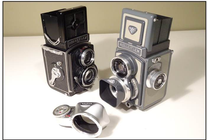
Two examples of "Baby" Rolleiflexes taking 127 film. Camera on Left: the 1938 "Sport" had an f/2.8 Zeiss taking lens and film advance crank. Camera on Right: the 1965 Grey Baby with f/3.5 Schneider lenses was marketed to ladies, travelers and "super slide" shooters.
