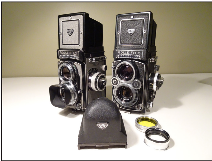
Camera on Left: Rolleiflex T (for Tessar) ca. 1961 with EV shutter and uncoupled meter. Camera on Right: Rolleiflex 3.5F ca. 1968 with Prism finder attachment and close-up lenses.
