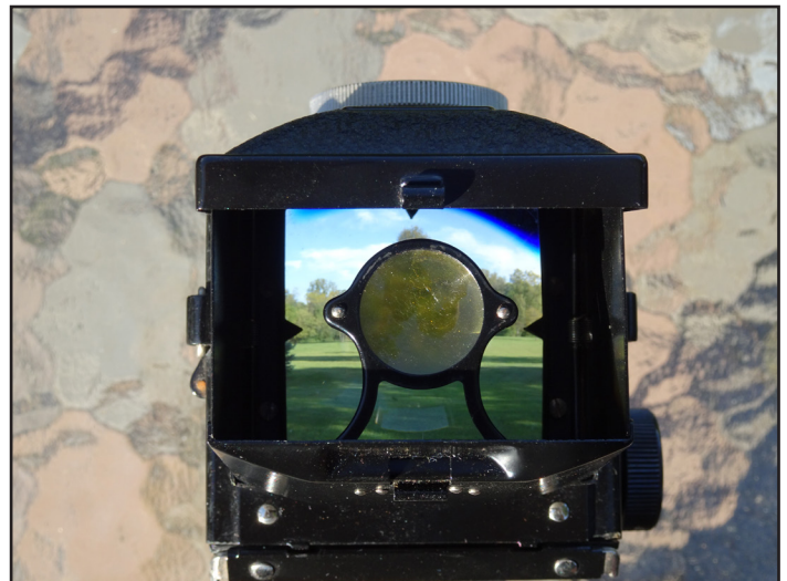
Viewfinder open with focusing spot erected. Notice the brilliance of the viewfinder unhampered by a stationary ground glass focusing screen.
