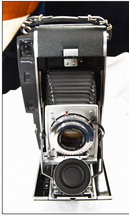
The professional Polaroid 110 with Tominon optics and Synchro-Compur shutter.
