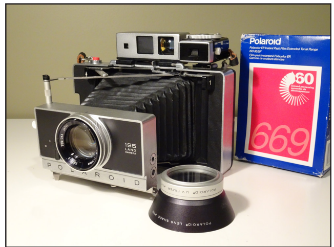
The Pack Film version of the professional 110 called the 195, shown with CdS exposure meter.
