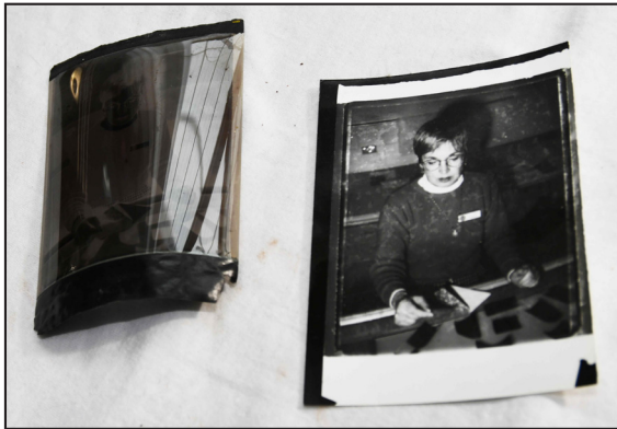
Polaroid even had pack film that produced a printable high resolution negative along with a B&W print. (Type 105).
