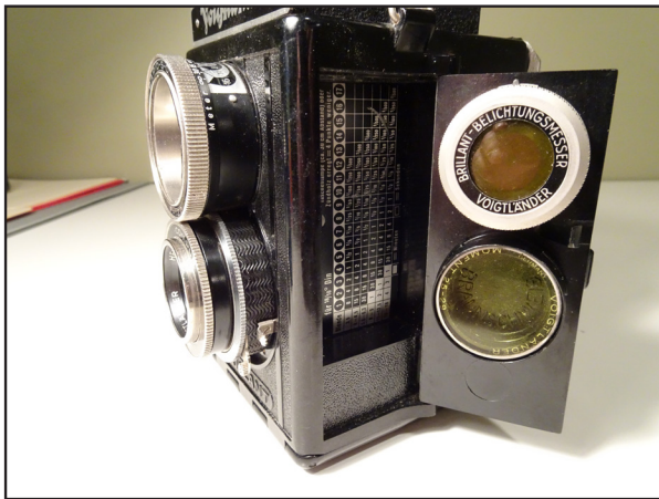
The V6 (Bakelite) Brillants had a secret accessory door in the side of its body containing a yellow contrast filter and an extinction meter. The exposure chart inside was for use with this early meter type and appears to be relatively accurate for early film speeds.
