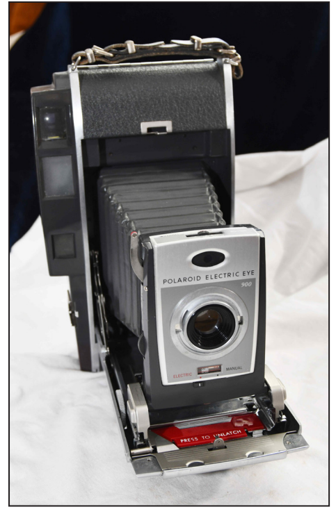
The innovative Polaroid 900 with "Electric Eye" auto exposure.
