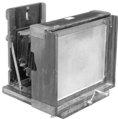
FIGURE 6. Rear view shows the folding focusing handle that is attached to an endless screw. Note the cutout in the rear assembly for the folding handle. The view also shows how the front bellows can be slid up and removed from the inner lens panel.
